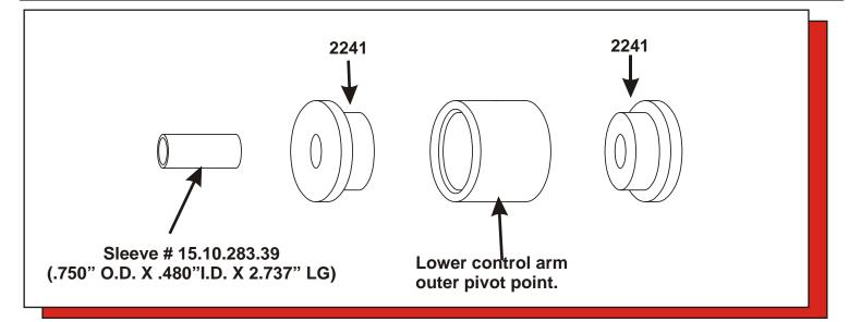
1. Remove the rear control arm from the vehicle.
